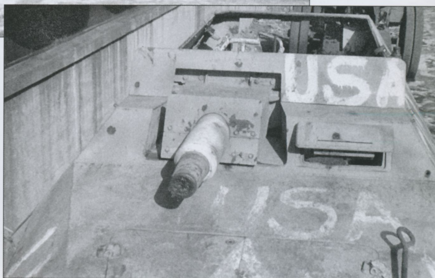
Another view of the 2.Panzer-Division Stummel providing a more detailed version of the original configuration of the 7.5cm howitzer mounting on the Sd.Kfz.251/9.
