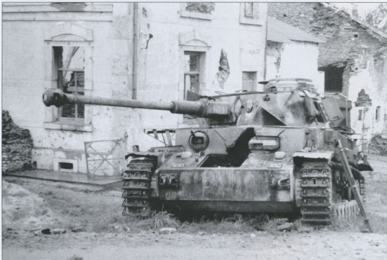
A Pz.Kpfw.IV knocked out in the fighting near Bastogne during the Battle of the Bulge and photographed the following summer. It has suffered a catastrophic failure of the front armor, probably a direct hit by an artillery round.
