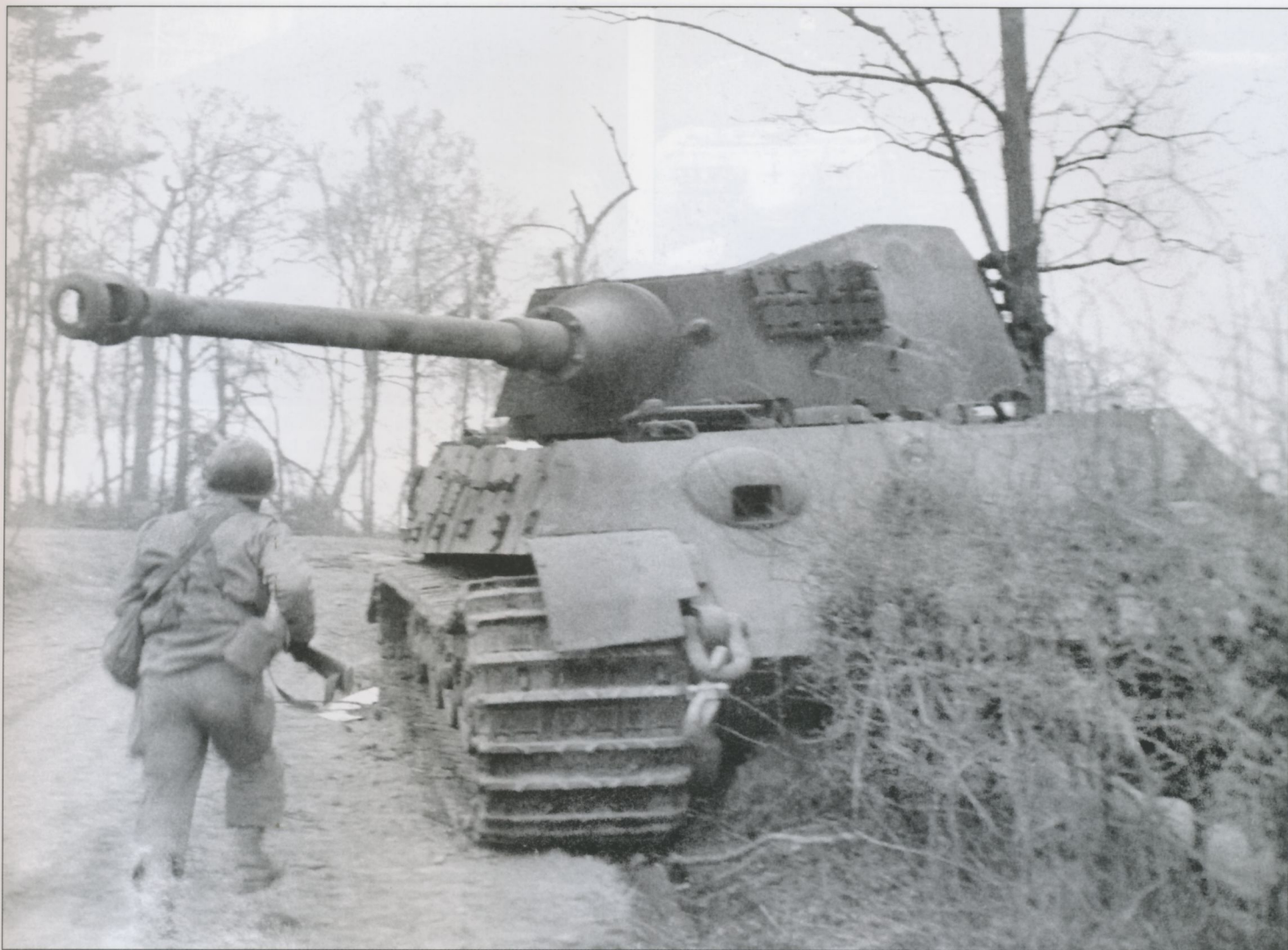
A US infantryman rushes by a knocked out Kingtiger near Weverousch, Germany on 27 March 1945. An internal explosion has blown off the turret roof.
