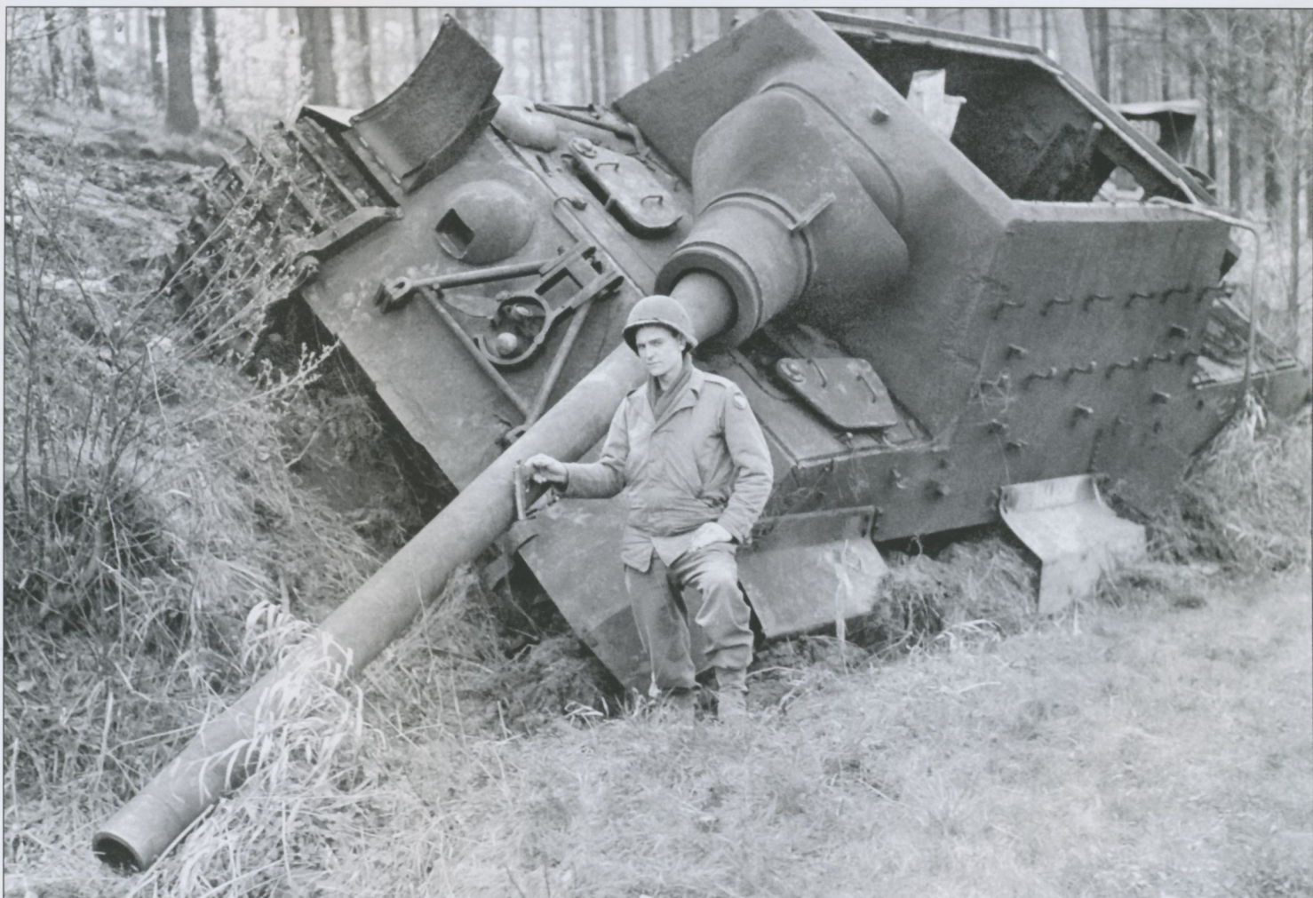
A Jagdtiger of s.Pz.Jg.Abt.512 claimed by a Sherman of the 750th Tank Battalion seen here after it was pushed off a road near Offensen, Germany on 9 April 1945. An internal ammunition fire has blown off the roof.
