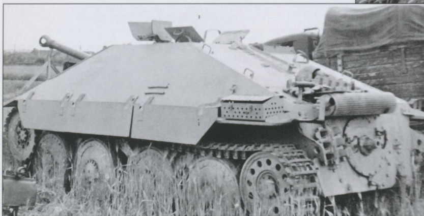
Another view of the Hillersleben Hetzer from the rear showing early production features.
