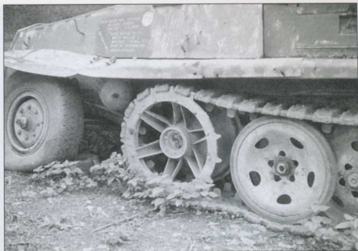
A close-up photo of the drive sprocket and suspension detail of Thorn.
