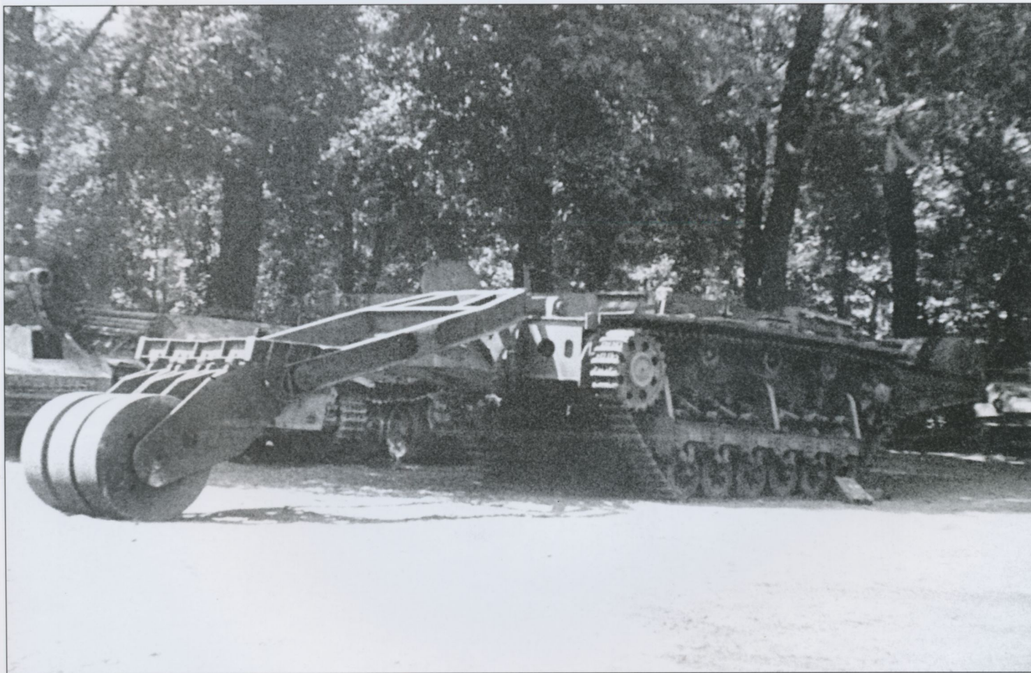
One of the rarer versions of the Pz.Kpfw.III was the Minenraumerpanzer III, an experimental mine-roller vehicle. One of the prototypes is seen here at a US Army ordnance holding area near Paris.
