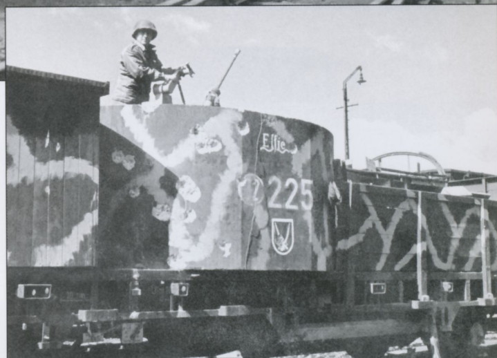
A GI looks over a 2cm flak cannon mounted in a concrete parapet for train defense on a train captured in Germany in April 1945. These types of protected mounts were used on armored trains as well as on regular transport trains for self-defense against Allied fighter-bombers.
