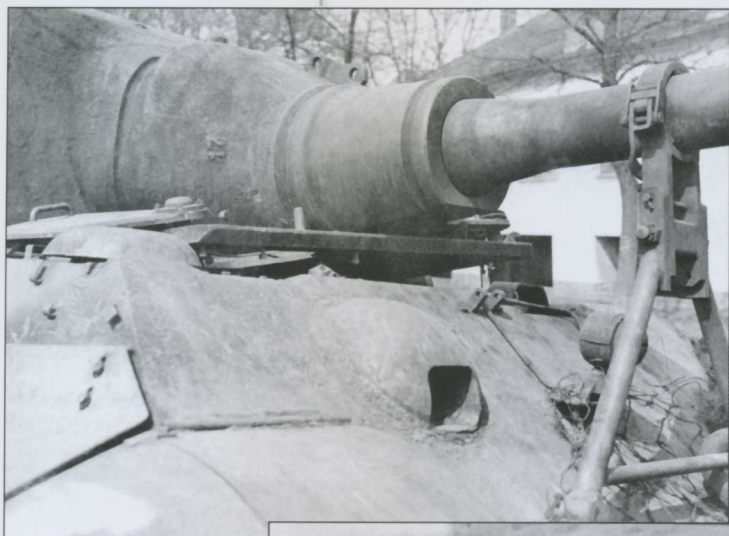
Another view of one of the Paderborn Jagdtigers showing a close-up of the mantlet and the heavy barrel travel lock.
