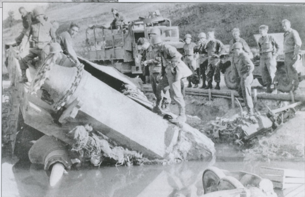
Another view of one of the Paderborn Jagdtigers showing a close-up of the mantlet and the heavy barrel travel lock.
