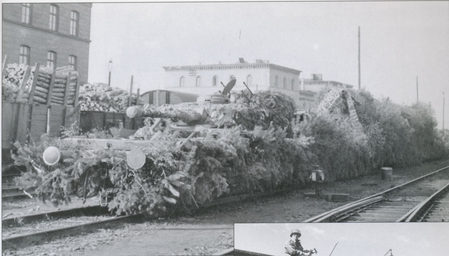
This shows the other end of the armored train armed with a flat-car mounting a Pz.Kpfw.IV turret.
