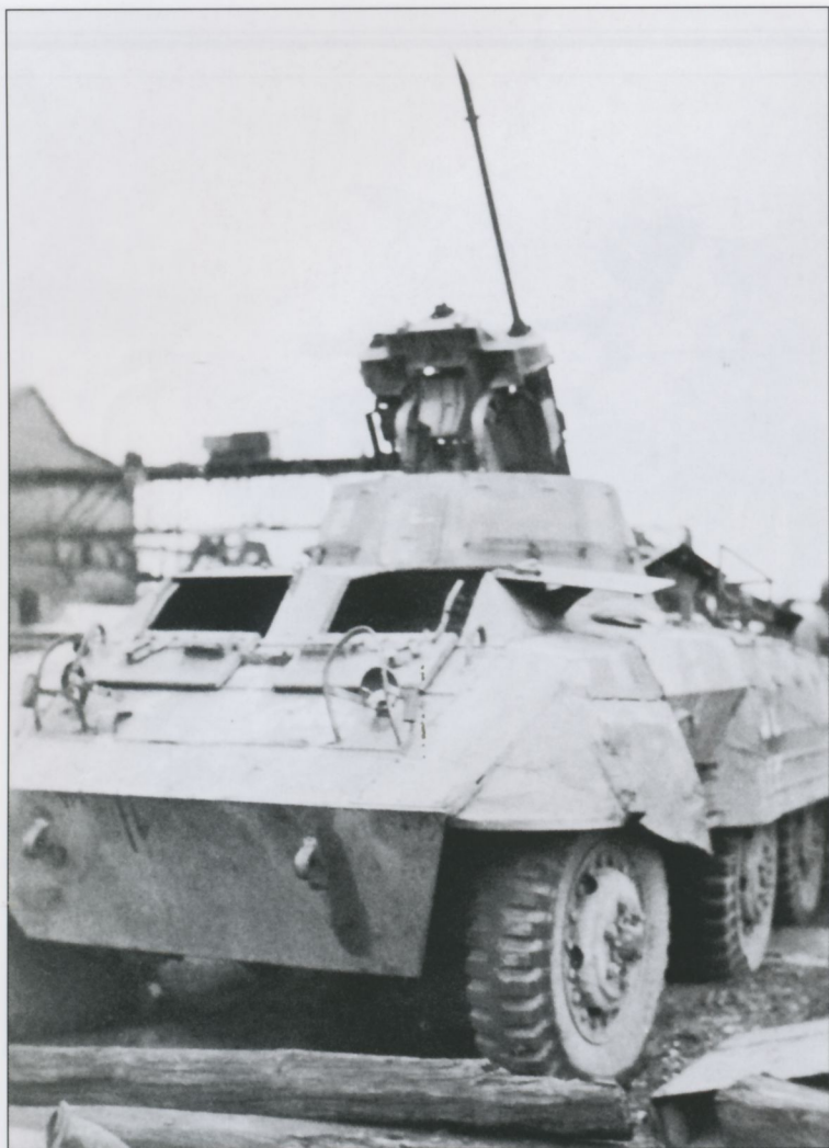
While captured US M8 armored cars were not particularly rare, this version certainly was. It has been reequipped with a 1.5cm Drilling anti-aircraft cannon mount instead of its usual 37mm gun.
