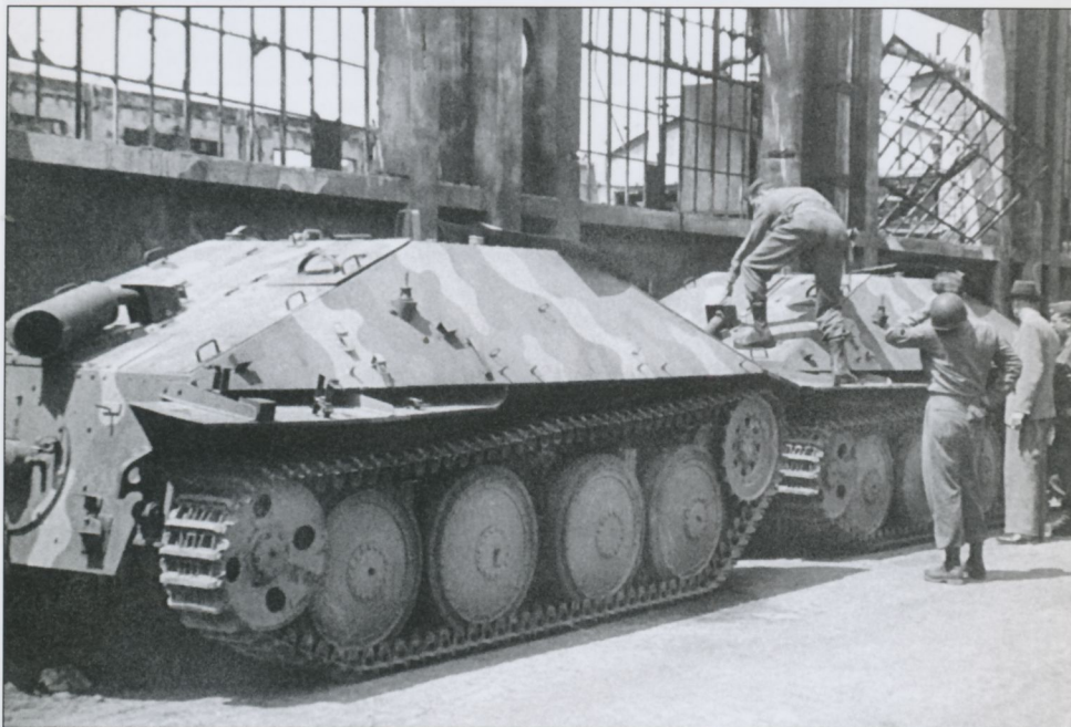
Another view from the Skoda assembly hall. One of the more curious features of the late production Skoda Jagdpanzer 38s was the painting of black rectangles near the view slits, presumably to create false targets.
