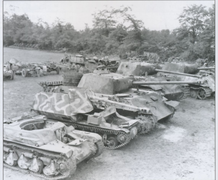
Another ordnance yard was created near Isigny at Trevieres in Normandy and this is a view of some of its holdings on 4 September 1944. Aside from the three Panther tanks, there is a Renault R-35 which had been converted to carry a 4.7cm anti-tank gun but with the superstructure subsequently removed. To its left is a Chenillette Lorraine converted into a tank destroyer with the addition of a 7.5cm PaK 40 anti-tank gun, and named Lowe (lion).
