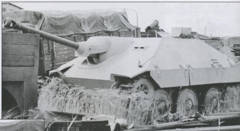
Another view of the Hillersleben Hetzer from the rear showing early production features.
