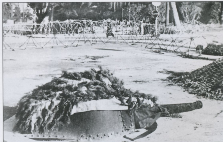
The obsolete Pz.Kpfw.38(t) turret was also widely used for coastal defense like this example near the coast in Marseilles.
