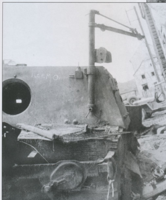
A detailed rear view showing the ammunition loading crane of the Duren Sturmtiger.
