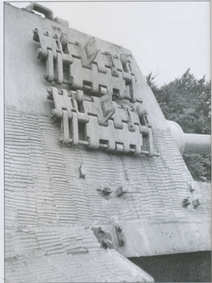
A detail view of the Haustenbeck Jagdtiger showing the spare track link stowage on the right hull side.
