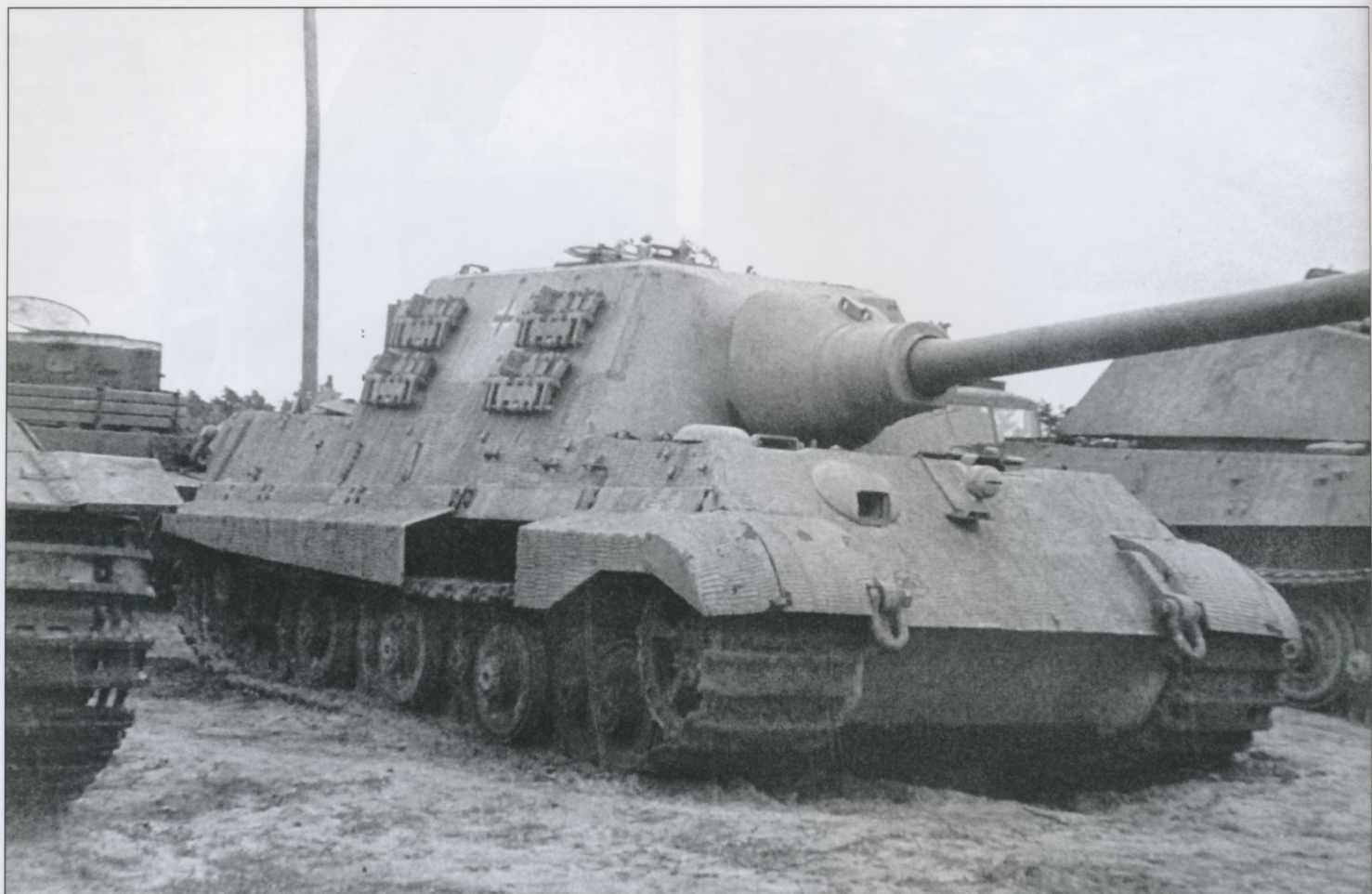
A US technical intelligence team after the fighting photographed this pilot Jagdtiger at the Henschel proving ground at Haustenbeck near the Henschel and Wegman plants in Kassel. It is one of the two initial vehicles built with the Porsche suspension.
